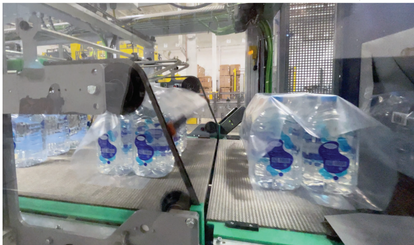
Multipacking in a Robopac shrink tunnel; no corrugated is needed. Clear film is pictured, but Cristalia recently employed decorated, registered film for a better appearance when the bottles are stacked as stand-alone displays (image on page 3).
