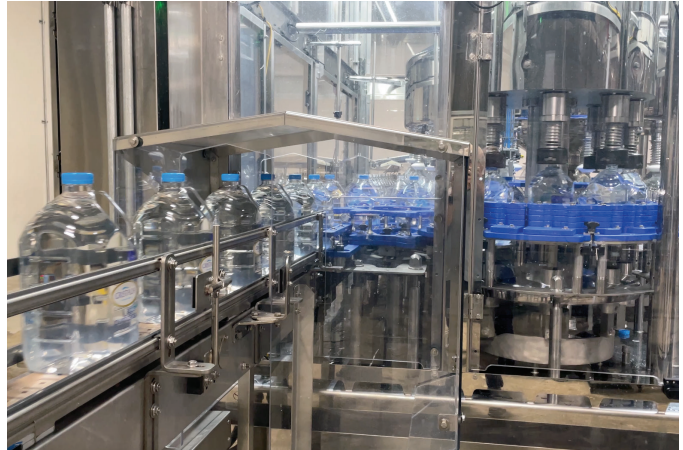
Bottles are filled on an eight-head monoblock filler from Fogg Filler, with capping (center right) immediately following.
