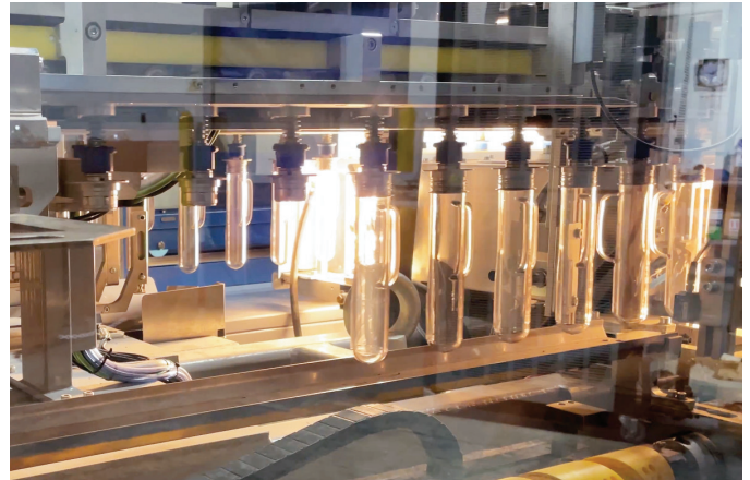
Preforms first travel into a five-cavity SIPA linear SFL blow mold machine, where they're blown at a rate of 83 bottles/min.
