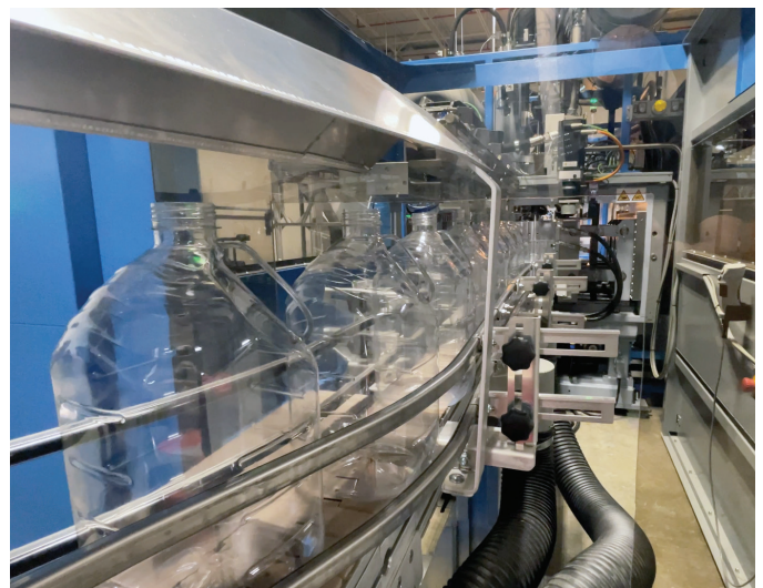
Blown bottles exit the blow molder on Dyco conveyers.
