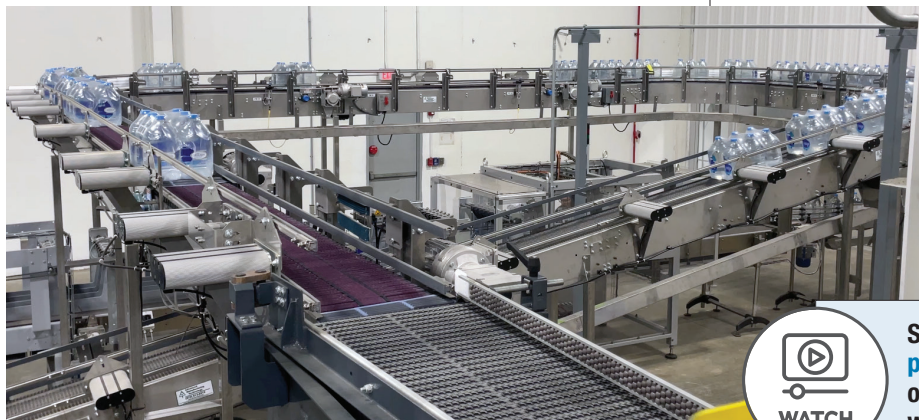
Shrink-wrapped multipacks flow to a palletizer via AMT conveyor.
