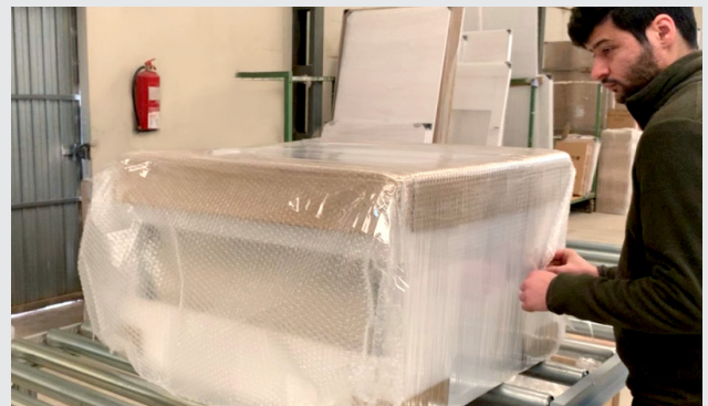
Product is wrapped in stretch and bubble film when coming out of the machine
